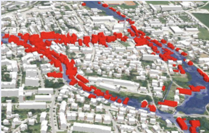
Figure 8. Examples of applications using CityGML models: 99 On the right, simulation of wind speed and turbulence effect of newly planned buildings; on the left, a flood scenario simulation and detection of buildings that will be affected according to this scenario.
